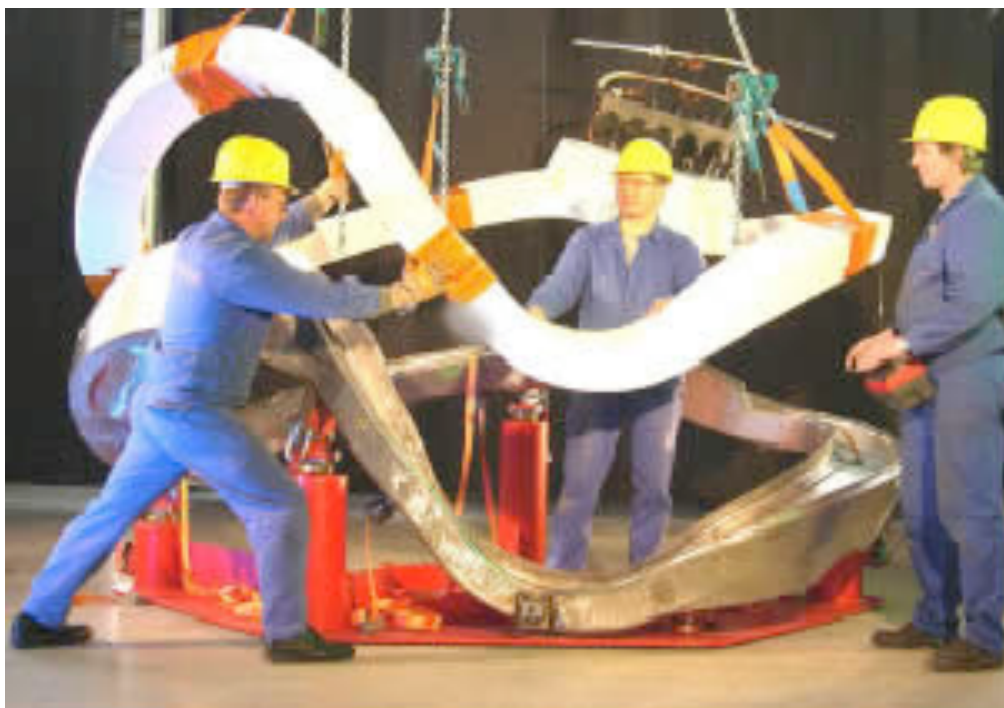
Wendelstein 7-X Stellarator magnets are complex
