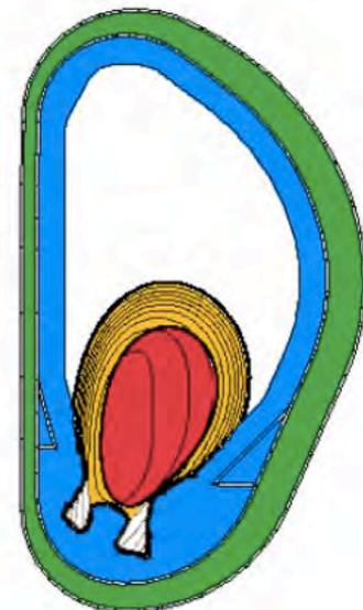
**Figure 4.3-2 Plasma Current Density during a Downward VDE**
