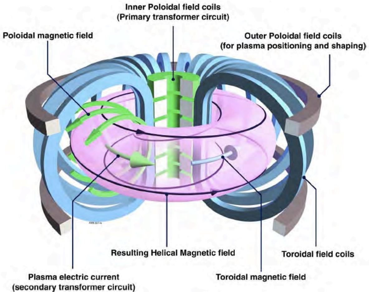
Figure 1.1: The tokamak [2]
