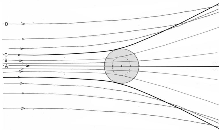
Fig.12 – Photon paths through the negative-mass object.
