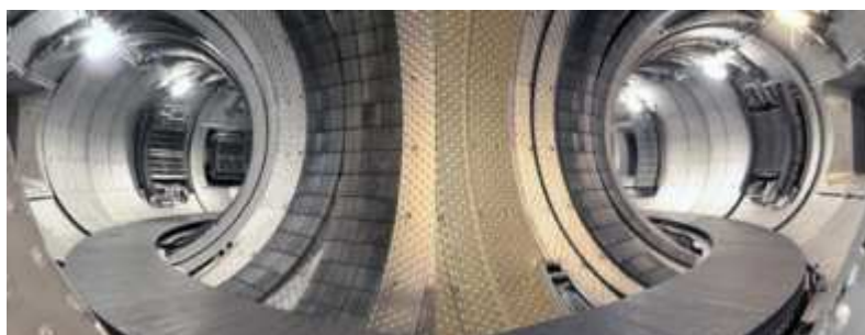
The chamber of Tore Supra. At the bottom, its “limiter”.
