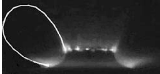
Fig2 : The electric discharge is blown away by the magnetic field gradient
