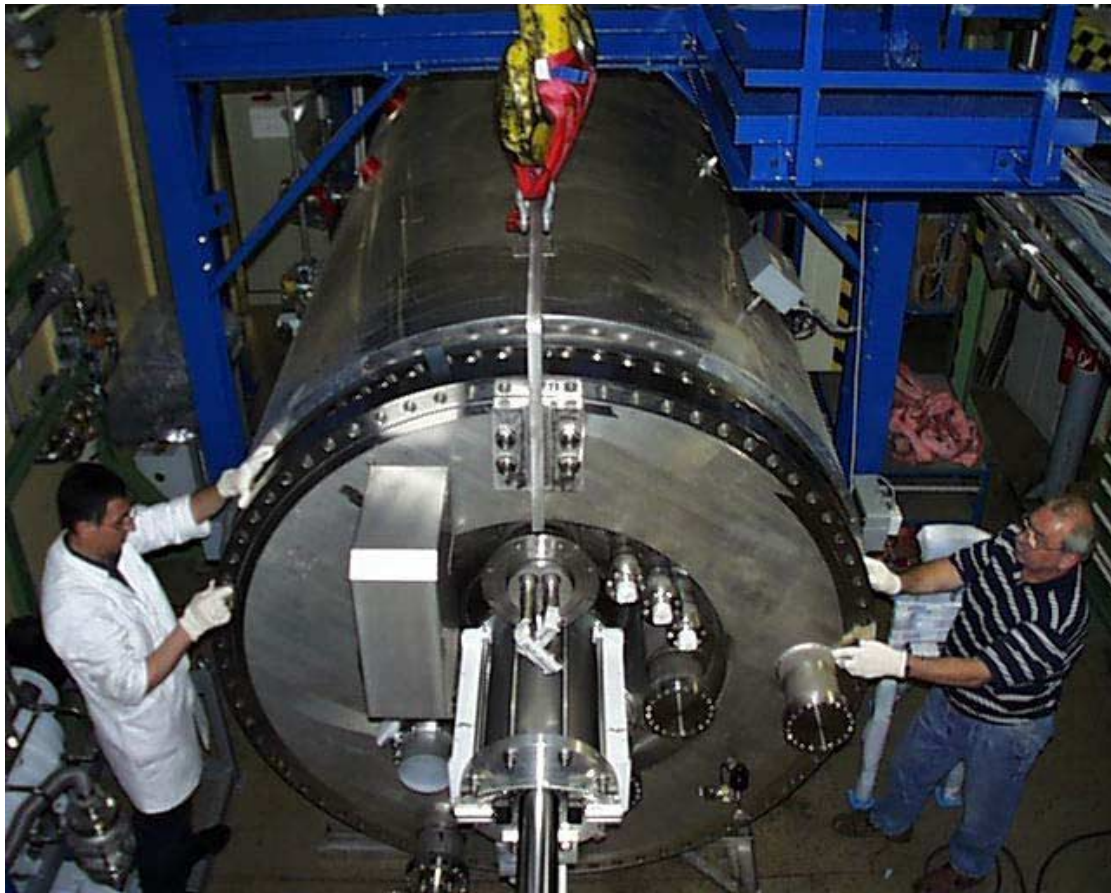
Figure 5.7-1 50% Scale Cryogenic Pump (EU)
