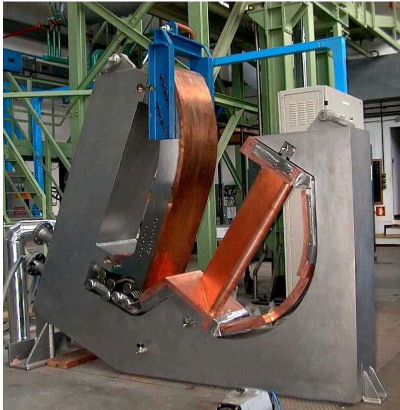
Figure 5.5-1 Integrated Outer Divertor Cassette (EU)
