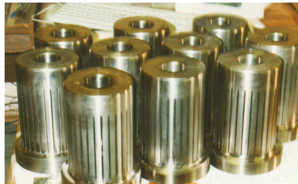
Figure 5.4-1 Flexible Mechanical Attachments made of Ti-Alloy (RF)
