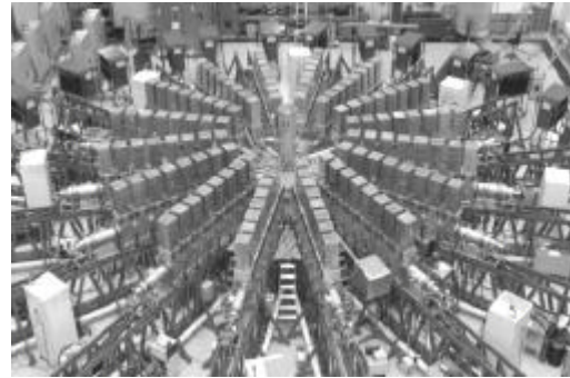
Fig. 1 : Sphinx machine, 16m diameter, 3m height 16 branches, 8 LTD-05 stages per branch
